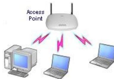
Fig. 6 WLAN access configuration using Access Point
